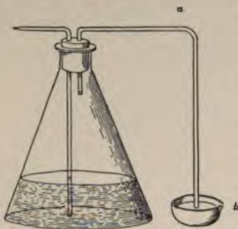
FIG. 28. — Flask arranged for culture of anaerobes which develop gas.
